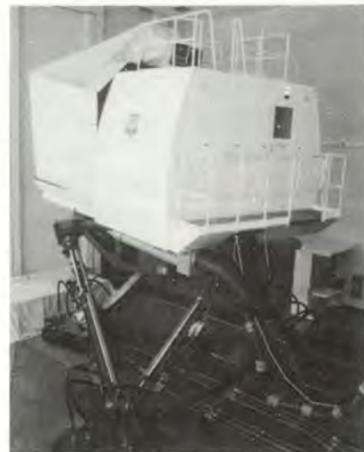
The motion base for the flight deck can move in six different directions: horizontal, vertical, lateral, roll, pitch, and yaw. The 18,000 pound flight deck can move 51 inches horizontally in less than two seconds. It can generate one half "G" of acceleration forward, zero "G's" downward, and two "G's" in an upward direction. Pitch can vary from plus 25 degrees to minus 29 degrees, a roll can be plus or minus 27 degrees, and yaw plus or minus 32 degrees.
