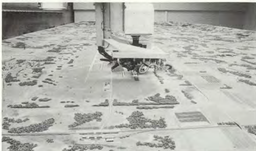
The terrain model is mounted vertically, measures 15 x 48 feet, and represents a hypothetical 5 x 15 mile terrain area. The camera moves on precisely aligned rails, horizontally and vertically, to represent aircraft position, and laterally for altitude.
